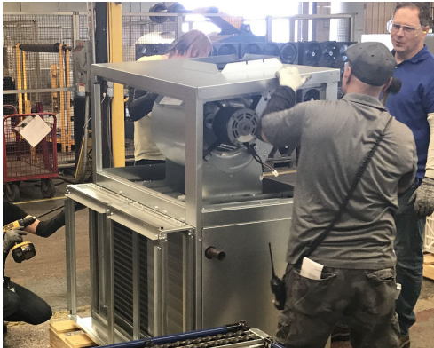
IEC team members working on final assembly of the new Vertical Direct Drive Blower Coils
